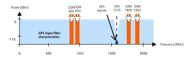
The MS32SN4 is configured with SAW to reduce out-of-band interference by adding a SAW filter.
