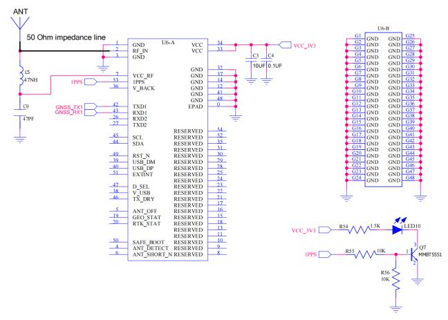
If the high-precision active antenna is a low-power design with 1.8V power supply, pin 8 can be used to supply 1.8V. Of course, the high-precision antenna can be externally powered, and when the antenna is externally powered, L5 47nH NC, change to an external power supply of 3.3V or other antenna-adapted voltage.
