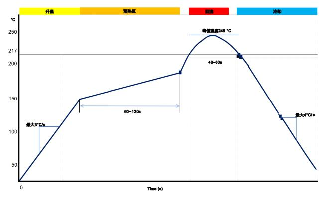
In order to prevent the module from falling off during soldering, please do not design the module to be soldered on the back of the board, and it is better not to go through two soldering cycles.
