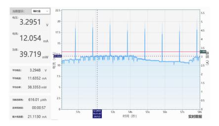
The measured data of the current in the dormant phase are as follows:
