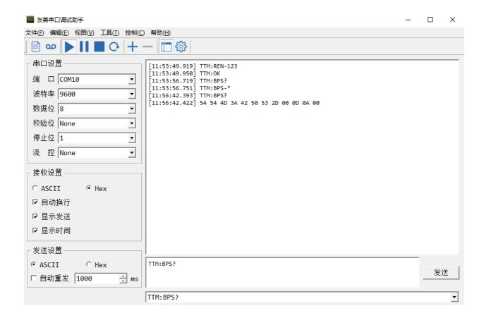
When querying device parameters, the values are in hexadecimal format. If ASCII display is selected, the parameter positions may appear as garbled text. In this case, you should set it to HEX display. The parameters will correspond to the positions after "2D" in the output. To check the baud rate, make sure to use HEX display to view the specific parameters.
